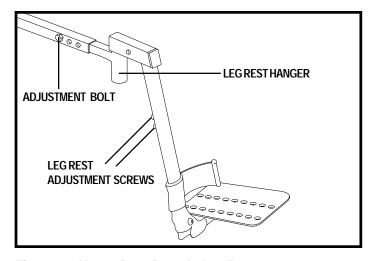
Figure 22. Heavy Duty Drop-In Leg Rests
